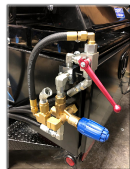
Mounted flow and Pressure Controls
